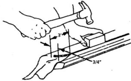
C. For side pockets, start approximately 3" from end of rail and pull cloth toward rubber cushion until the edge of the cloth is approximately 1/2" from the end of the feather strip. Tap feather strip in place.
