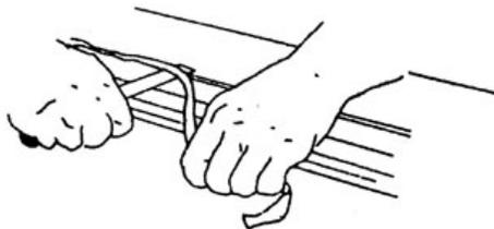
**NOTE:** IF FEATHER STRIPS ARE LOOSE ADD A STRIP OF MASKING TAPE THE FULL LENGTH OF STRIP.
