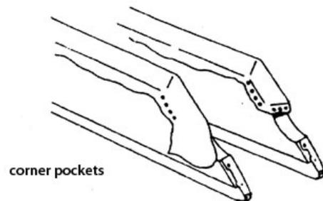
B. For side pockets, stretch cloth firmly over nose of cushion toward the bottom without distorting cushion shape. **Pull cloth tightly toward side pocket before tacking.** Staple cloth to rail bottom approximately 1" from pocket opening.
