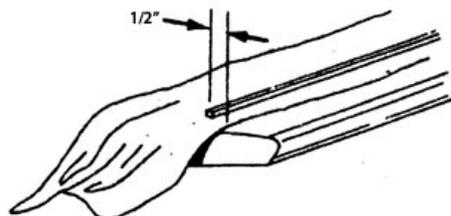
B. For corner pockets, tap feather strip in place except for 3" at each end. Start approximately 2" from end of feather strip and pull cloth toward rubber cushion until the edge of the cloth is approximately 3/4" from the end of the feather strip. Tap feather strip in place.
