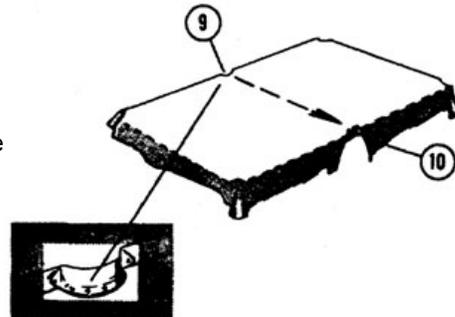
10. Stretching cloth tightly across the table from (9) repeat the above operation at (10). Be sure to tack cloth to undercut of slate frame.
