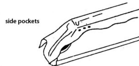
C. Snip cloth at nose and pull small strip down to groove. Staple in place as shown. Then snip (or fold) excess cloth leaving enough for small fold at the top as shown.
